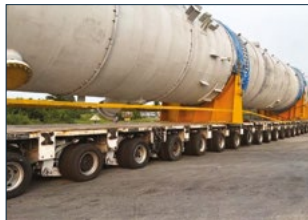
LHU Column being transported on an SPMT
