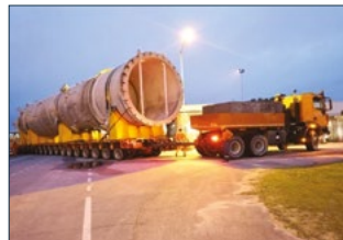
LHU Column being transported on an SPMT
